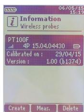
The probe information is displayed With the function key **"Meas."** It is possible to back to the measurement screen. It is also possible to delete the wireless probe pressing the function key **"Delete"**.
